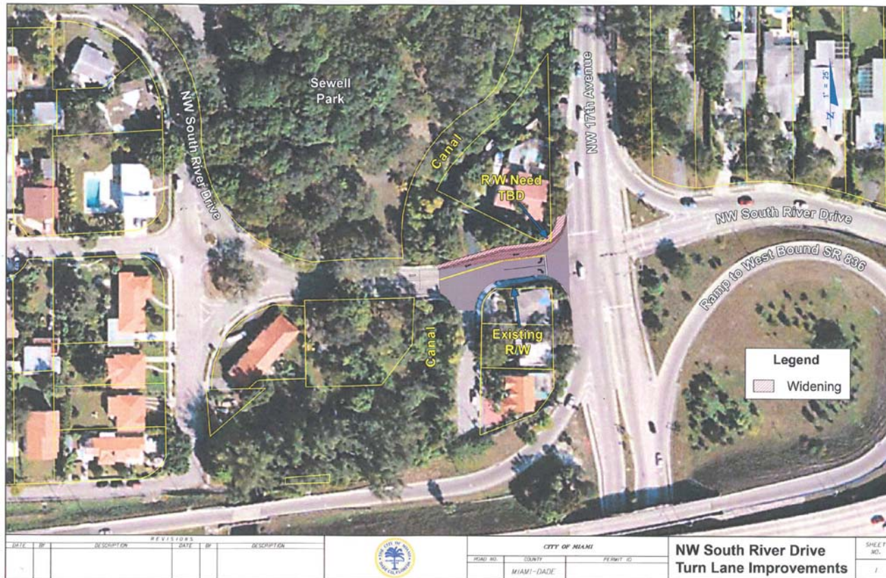
Schematic of Intersection Improvements at NW 17 th Avenue, NW 11 th Street and NW South River Drive
