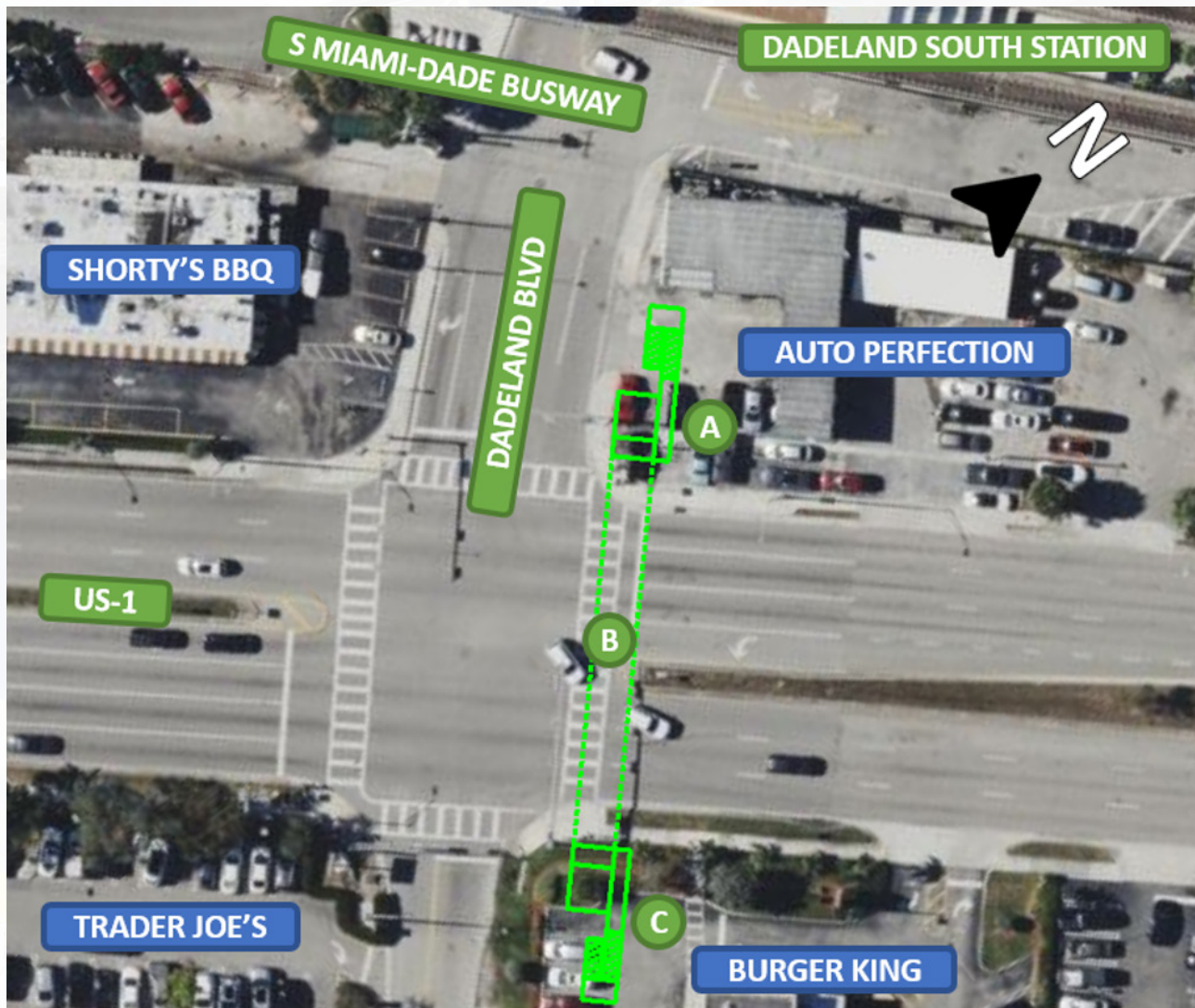
Figure 5-13: Dadeland South Metrorail Station Alternative 1: Pedestrian Bridge a Dadeland Boulevard
