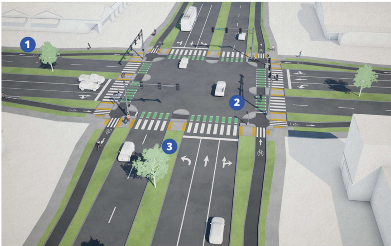
Figure 4-1 FHWA Protected Intersection Example
