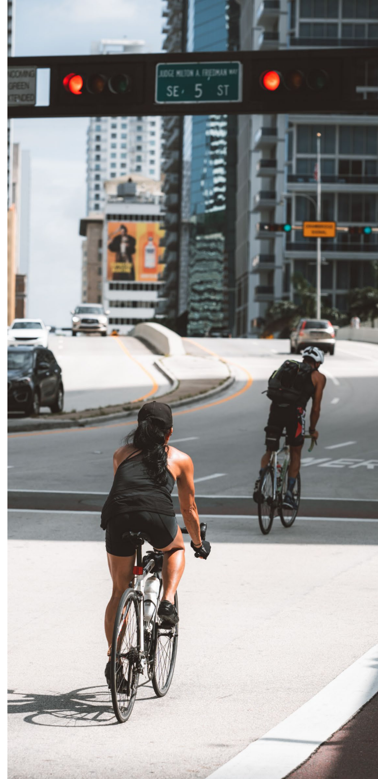
Figure 27: Cyclists travel through the intersection at Brickell Avenue and SE 5th Street, where the roadway transitions from a shared-lane marking to a dedicated bike lane.
