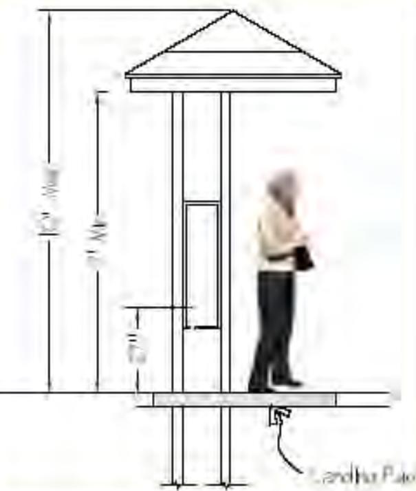
Fig 1.23 | Cross-section of a small bus shelter with a leaning rail but no seating, with typical vertical dimensions.
