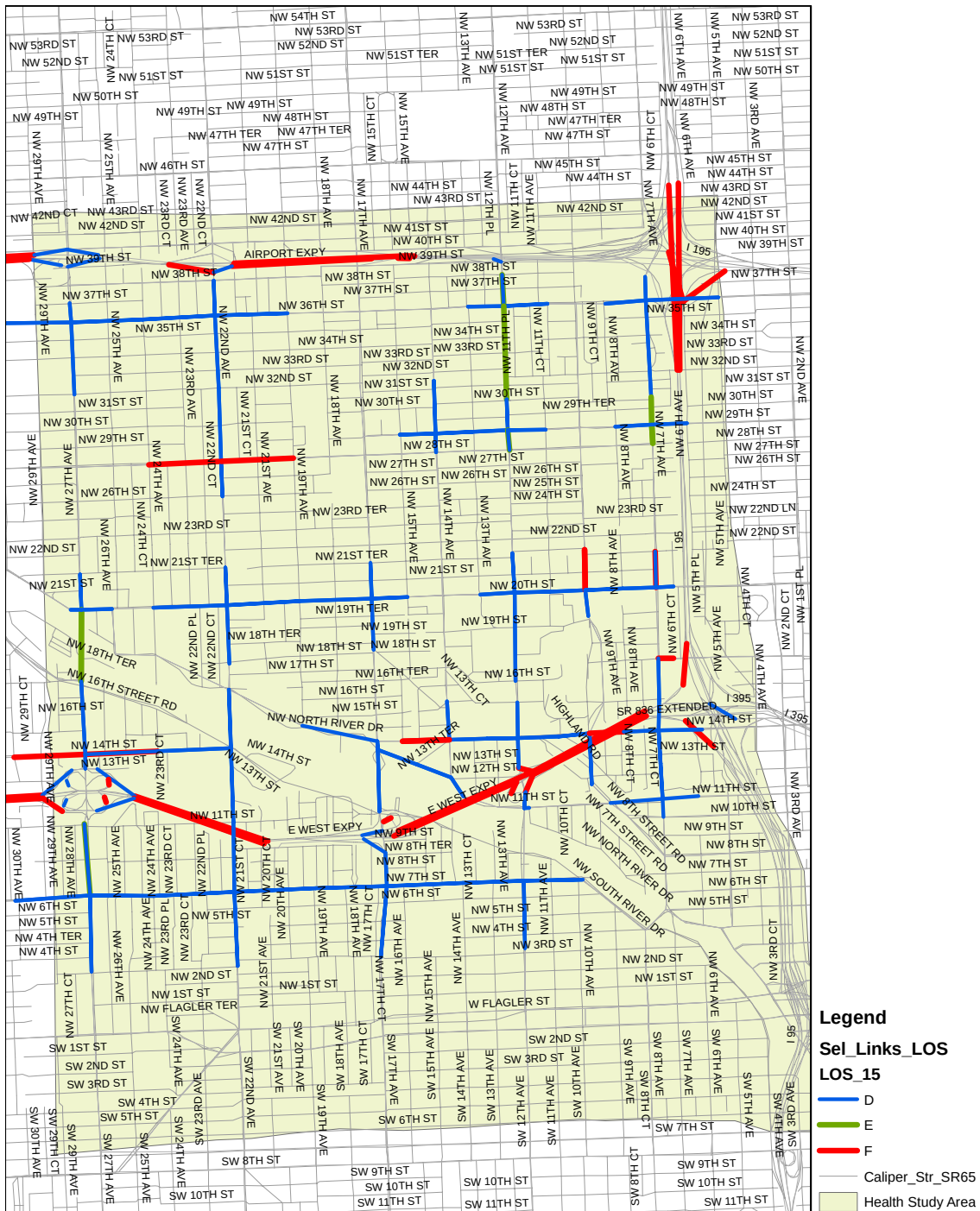
Figure 35: Deficiency Analysis for Year 2015 using Post Processed Results
