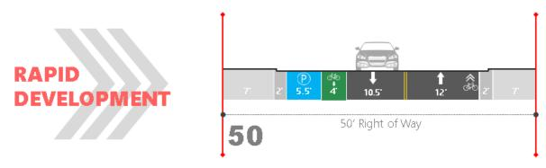
Figure 53: Rapid Development Alternative for 50' Typical Section
