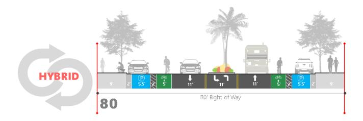
Figure 54: Hybrid Alternative for 80' Typical Section
