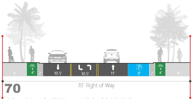
Figure 61: Situational Alternative for a 70' ROW incorporating bike lanes flushed with sidewalks.
