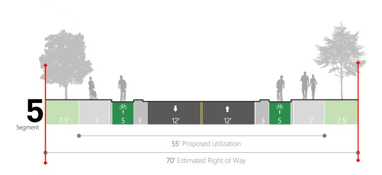
Figure 70: Pilot Project B – Proposed Typical Sections
