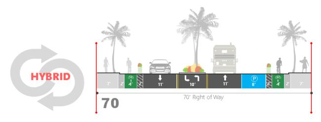
Figure 55: Hybrid Alternative for 70' Typical Section
