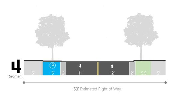
Figure 66: Pilot Project A – Existing Typical Sections
