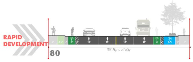
Figure 51: Rapid Development Alternative for 80' Typical Section
