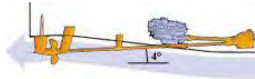
The Servogear System's Shaft Angle
