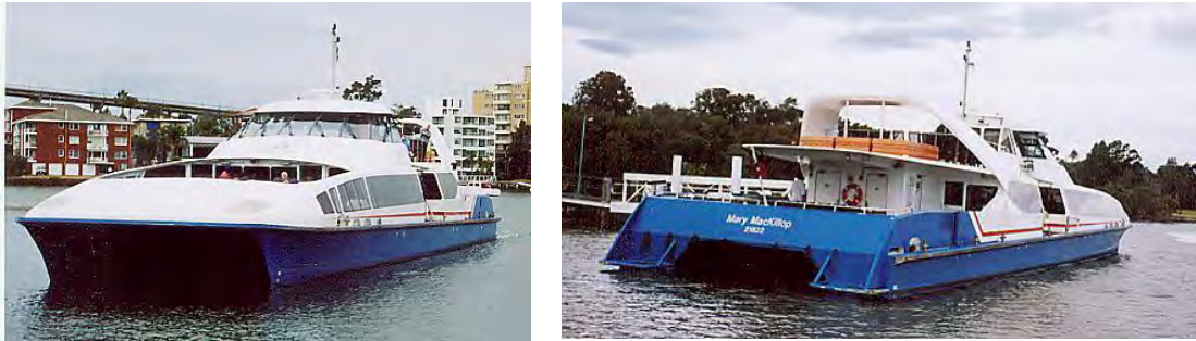
Exhibit 28. Aluminum Hulls and Composite Superstructures for Low Navigational Drafts
