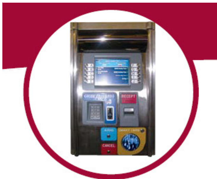
FIGURE 44: EXAMPLE OF A TVM (ELECTRONIC TRANSACTIONS ONLY) Source: cubic.com
