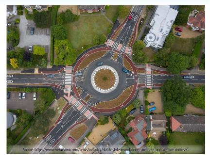
Figure 29: Modern roundabout ('Dutch' style) provides safe mobility and access for those driving, biking and walking.
