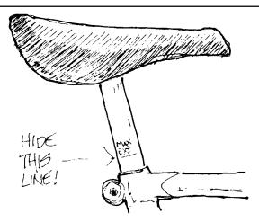
**Caution:** At least two inches of both the seat post and the handlebar stem should be inside the frame. Look for a mark with something like "MAX EXT" (maximum extension) next to it. That's your limit.
