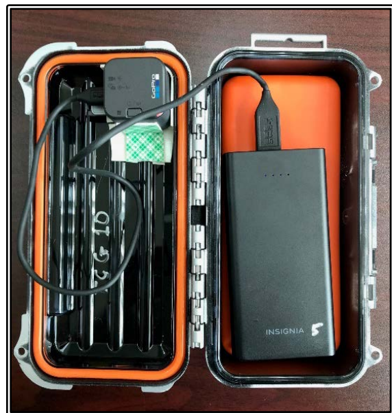
Data collection weatherproof video camera shown open with auxiliary battery and 200 GB SD memory chip installed (not visible)
