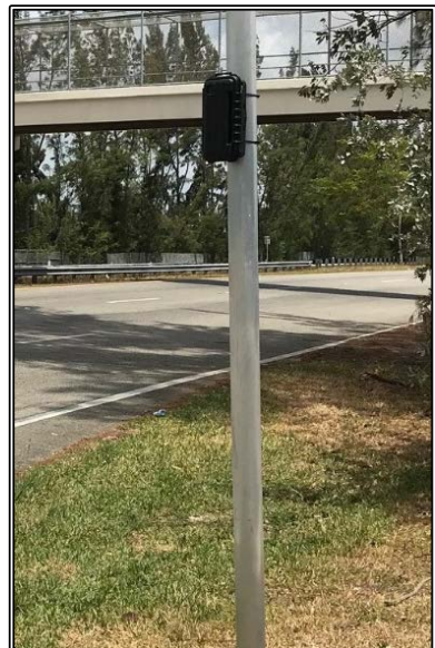
Data collection video camera mounted on S.R. 9 sign post with view down path
