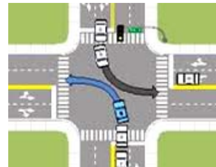
(Left): Turning radii are important at intersections; here, the diagram demonstrates spatial clearance in a turn. Issues arise with extended turn radii for trucks due to intersection design, as this may affect opposing vehicular and bicycling traffic making a turn.
