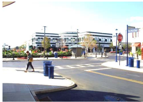
Bulbouts are curb extensions which can serve as neckdowns for traffic, and can be utilized to shorten crossing distances for pedestrians (Columbus, OH - Top Right). With innovation, they can also provide a rest area in a mini park, where people can sit (Keene, NH - Top Left), and city beautification, making walking a more enjoyable experience (Davis, CA - Bottom Left). Source: http://contextsensitivesolutions.org/
