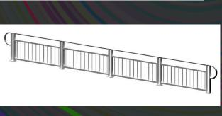
Where the path is adjacent to canals, ditches, or slopes steeper than 1:3, a wider separation should be considered. A minimum 5 foot separation from the edge of the path pavement to the top of the slope is desirable. Depending on the height of embankment and condition at the bottom, a physical barrier, such as a railing or chain link fence may need to be provided.
