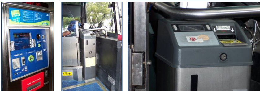
Illustrations of the Easy Card dispensing machine and the fareboxes installed at all buses.
