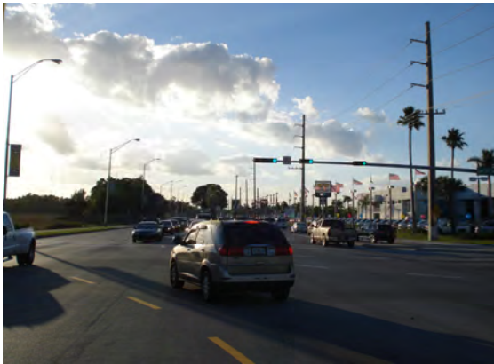
Westbound approach: Sight distance obstruction to left-turn traffic.
