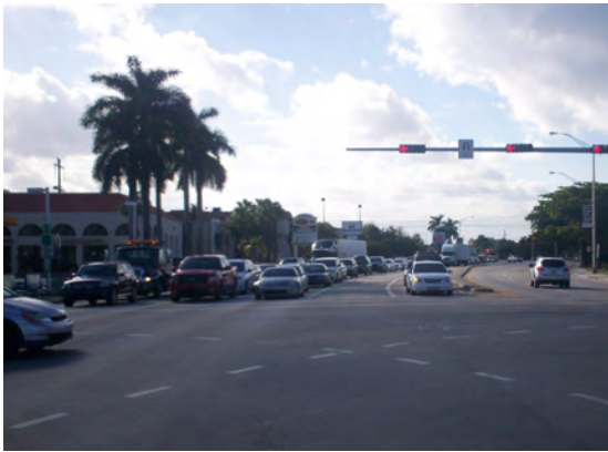
Eastbound approach: A large wide gore that can be converted to an extra lane.
