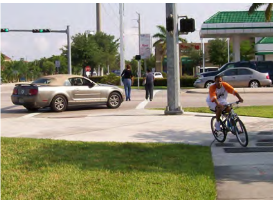
East leg: Pedestrians find it difficult to cross long crosswalk with insufficient time.
