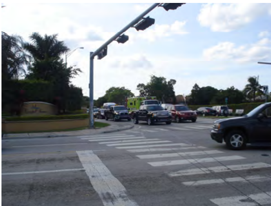
Northbound approach: Sight distance obstruction to oncoming traffic.
