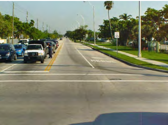
North leg northbound: Merging conditions with no warning signs.
