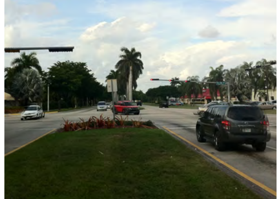
Eastbound/Westbound: Left-turn lanes are not aligned to reduce the offset.
