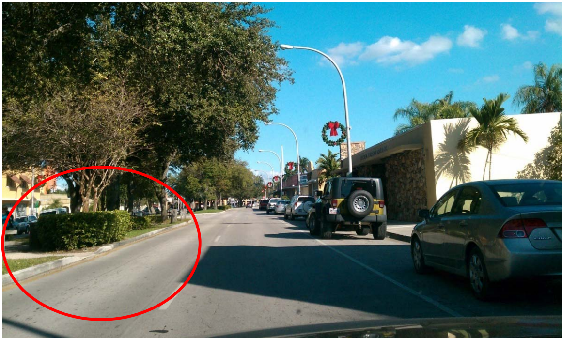
Eastbound on Westward Drive, just east of Park Street – Notice the pedestrian pathway in the center median that lacks connectivity to crosswalks at the intersection.
