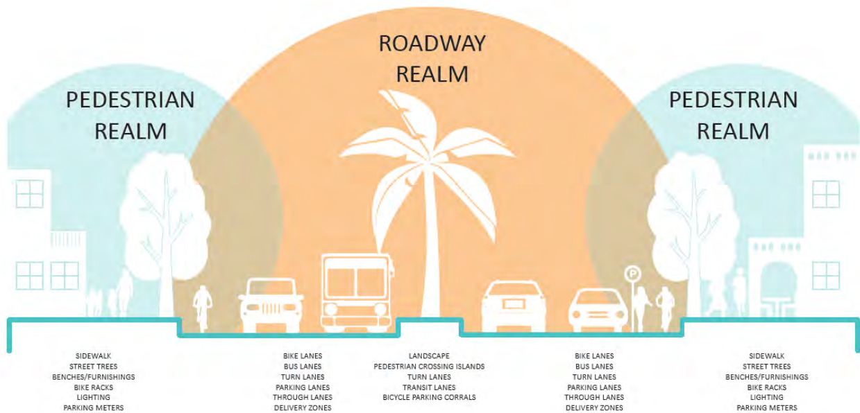
Figure 6: Complete Street Cross Section Elements
