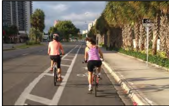
Figure 10: Buffered Bike Lane - Striping
