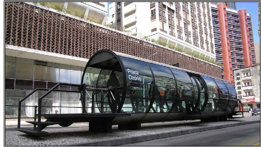
Bus Rapid Transit Raised platform bus stop that provides greater visibility, and the level-boarding platform improves passenger comfort and reduces stop delay time
