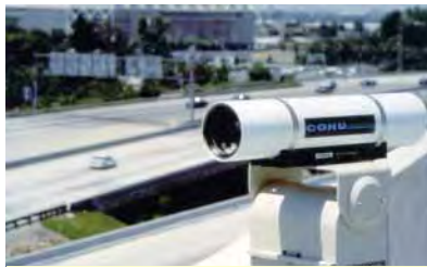
ITS cameras assist with real-time adjustments to the traffic signal system.
