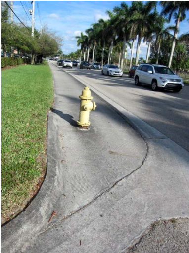
Observed sidewalk obstructions include utility poles in the middle of the sidewalk, with additional cables blocking the path for an alternate route (Top Left, Image source – Google Earth), Utility boxes and fire hydrants in sidewalks (Top Right), traffic signs (Bottom Left), and fire hydrants in sidewalks at curb areas (Bottom Right), all of which present issues for pedestrians, and some of which are non ADA compliant.
