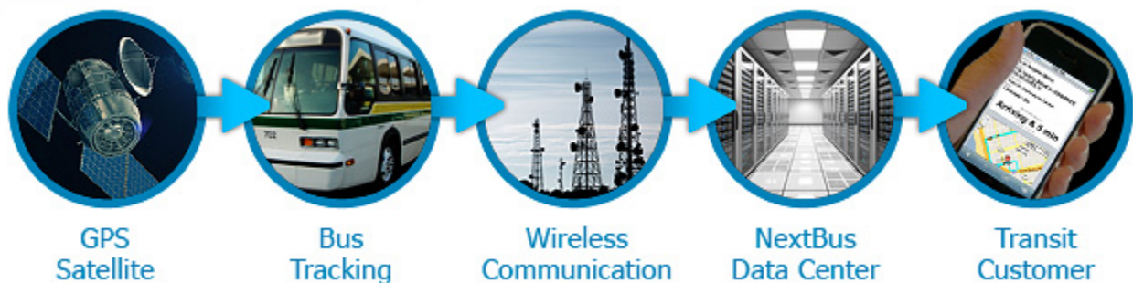
Figure 7-3 - NextBus Passenger Information System Information Flow
