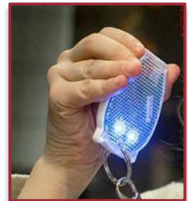
When a pedestrian is approaching a dangerous crossing the reflector—which features sensors, LED lights, wireless charging, and communications—can be made to blink and alert car drivers.
