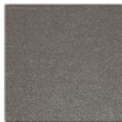
GRANITE TILES OPUSTONE BLACK ABS FLAMED FINISH FLOOR AT PLATFORM
